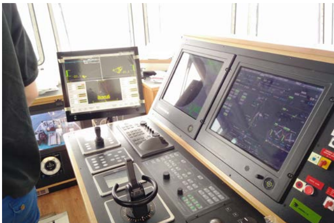
Implementation of the system on the bridge of the water injection dredger.
